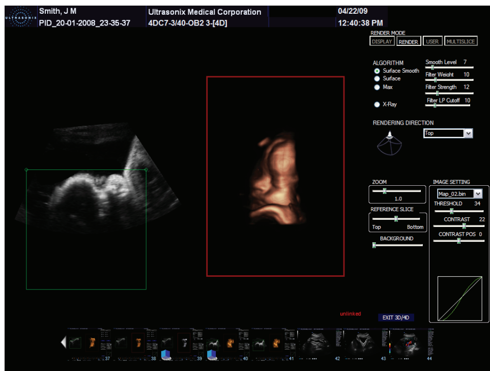
Figure 5-23: Render Mode LCD Display Options
